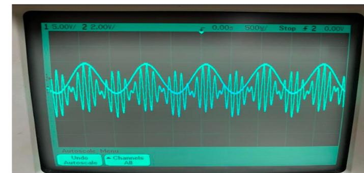
Fig. 4 MQQ Ssignal represented in the modulated signal.
