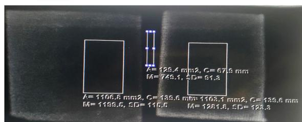
X-ray images of 0% SiC/polymer is shown on the right and 0.9% of SiC/polymer is shown on the left. Absorbed x-ray intensity and background noise are shown in the ROI's.
