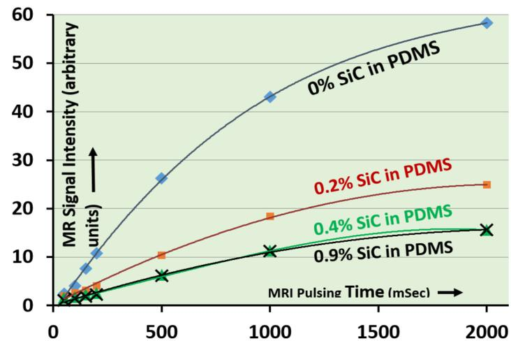
Fig 2 shows the increasing difficulty for PDMS to generate MR signal from the polymer when SiC is increased from 0-0.9%
