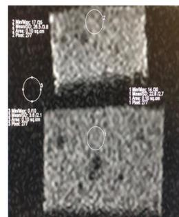
Fig 1 shows Signal/Background Noise for pure PDMS (Top) =  $(26.5-3.8)/2.1 = 10.8$  while that for 0.2% SiC filler PDMS Signal/Noise (Bottom) drops to  $(22.8-2.7)/2.1 = 9.6$ ; a 12% decrease, even 0.2% SiC impurities restrict polymer chains from freely moving. MR signal depends on mobility of molecules.
