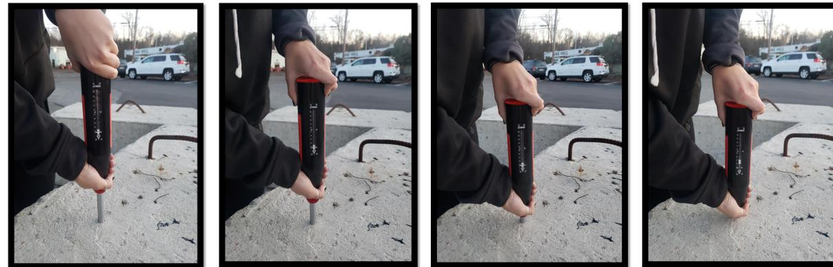
The above images represent the process of taking a reading from a Humboldt Schmidt Hammer.
