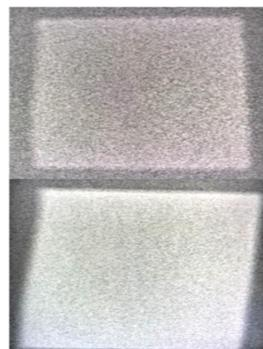
PDMS + 0.2 % SiC (top) low x-ray techniques (40kV, 1 mAs), and (bottom) is medium power X-ray 45kV, 10 mAs, no grid, 10 magnification. Low power x-ray image appears noisy (quantum mottle).
