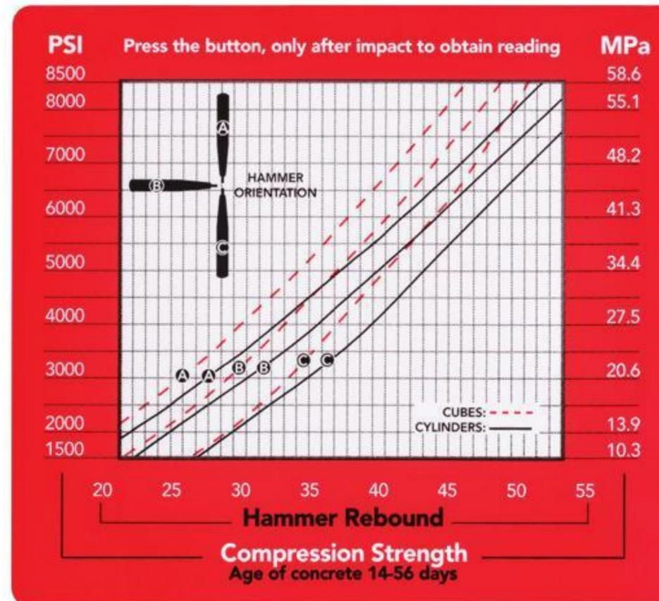
Depending on the position in which the test was taken, in this case Class A, the hammer rebound helps to determine the compressive strength in either PSI or MPa.
