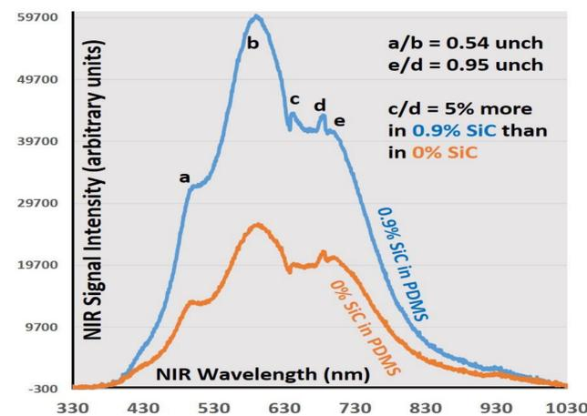
Fig 3 shows Near infra-red spectrum of 0 and 0.9% SiC fillers creating signature peaks between 600 and 750 nm wavelengths.
