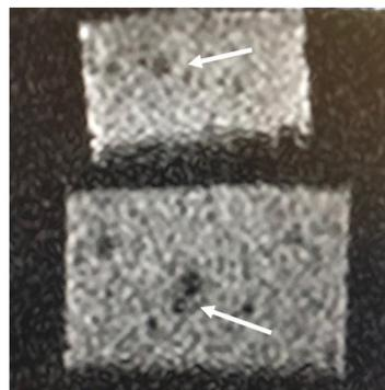
200 um resolution MR image (from Prisma 3T) Of 0% SiC/PDMS (top); 0.9% SiC/PDMS (bottom). Defects (white arrows) are approximately 1-2 mm in size (1000-2000 um)
