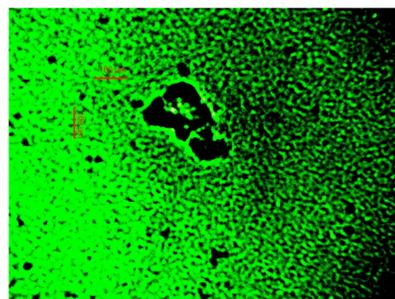
Fig 4 is a light microscopy image at 50x mag. showing a 300 um (0.3 mm) size defect in PDMS with 0.9% SiC.
