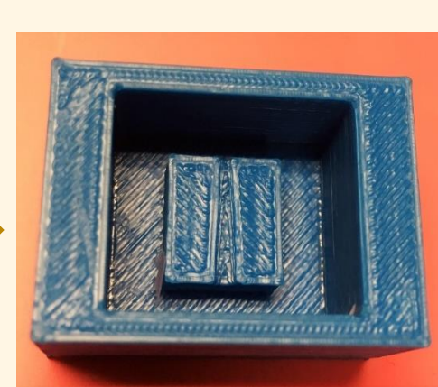
Fig. 2 3D scaffold mold printed on MakerBot printer
