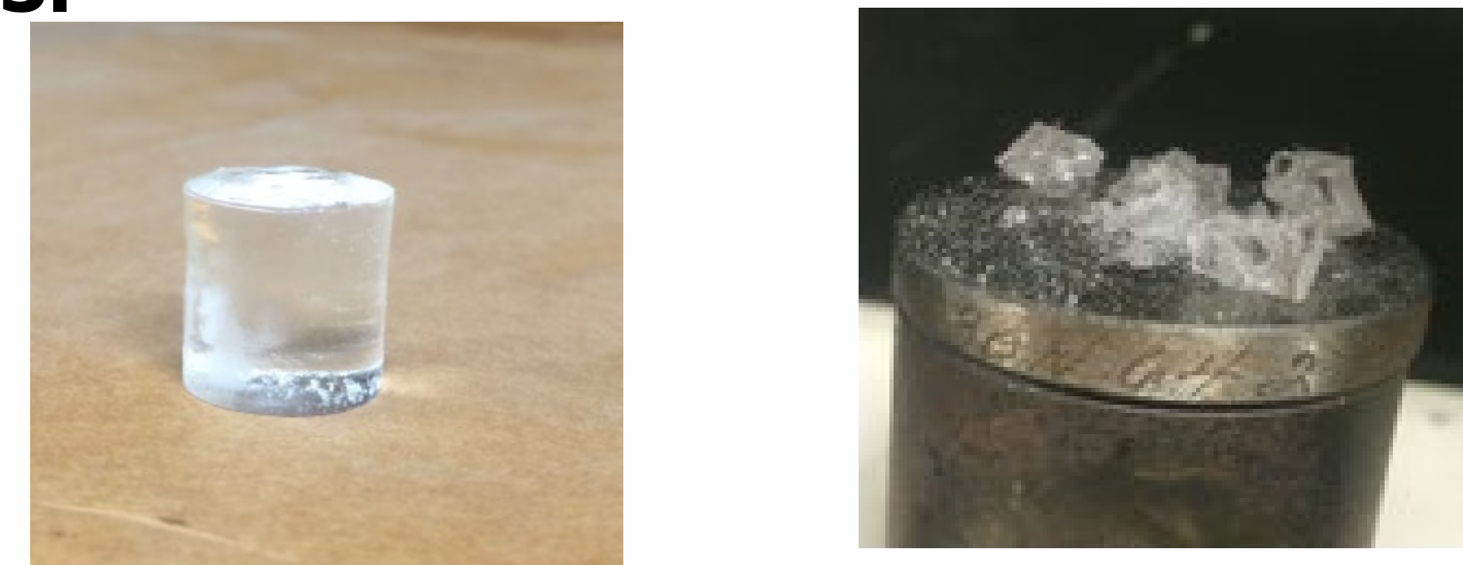
Fig 4. 3D Photopolymerized PEGDA before and after the compression test
