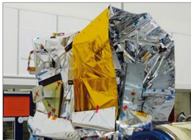
Thermal H/W (Radiators, Thermal Straps, MLI, etc)
