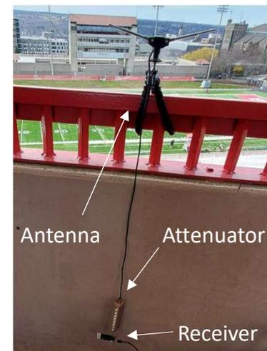
Figure 45: Receiver setup
