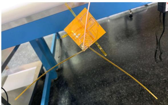
Figure 39: ChipSat suspended for antenna analysis
