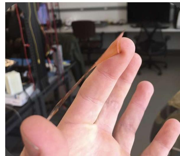
Figure 30: Side view of thin polyimide ChipSat PCB (no components soldered on)
