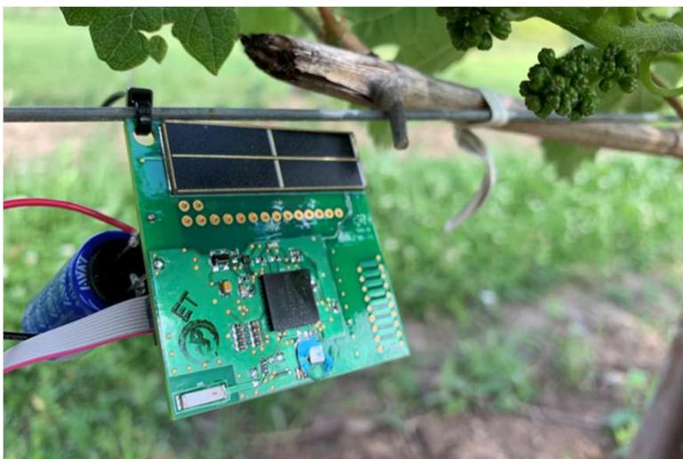
Figure 28: Helical antenna ChipSat on thicker FR4 substrate
