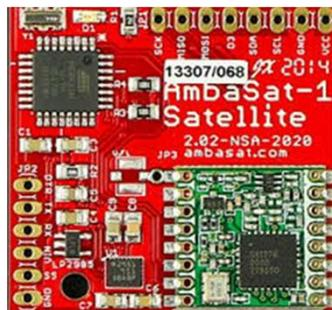
Figure 18: AmbaSat [5] (LoRa Module)
