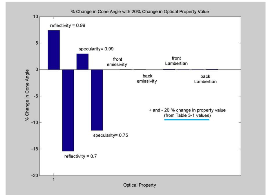
Relative Effects of Optical Properties on Sail Thrust Direction
