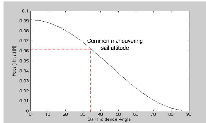
Solar Sail Total Force (Thrust) Vs. Sun-Incidence Angle
