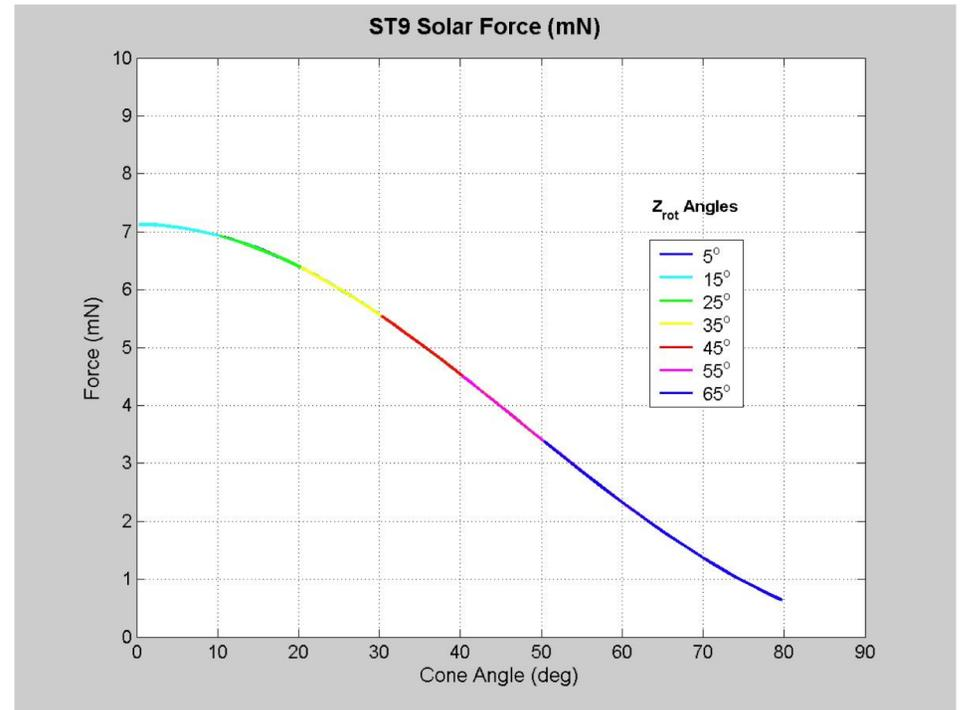
ST9 Thrust vs. Cone Angle Curve from "Simulated" Orbit Measurements
