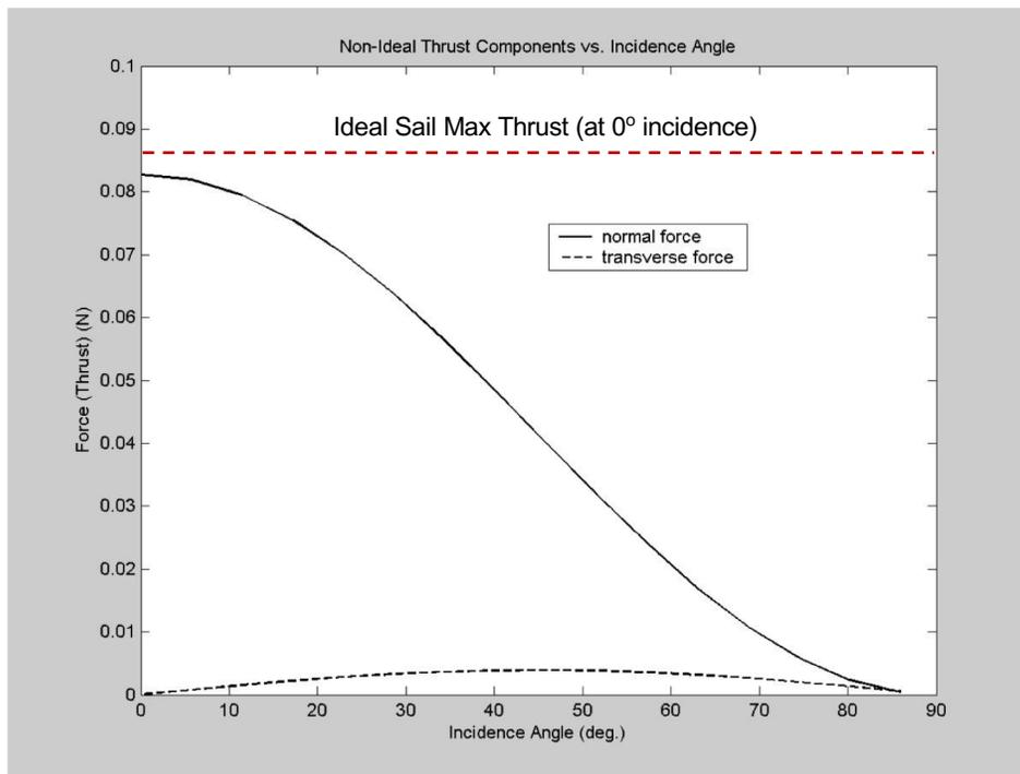
Normal and Tangential Force Components Vs. Sun-Incidence Angle
