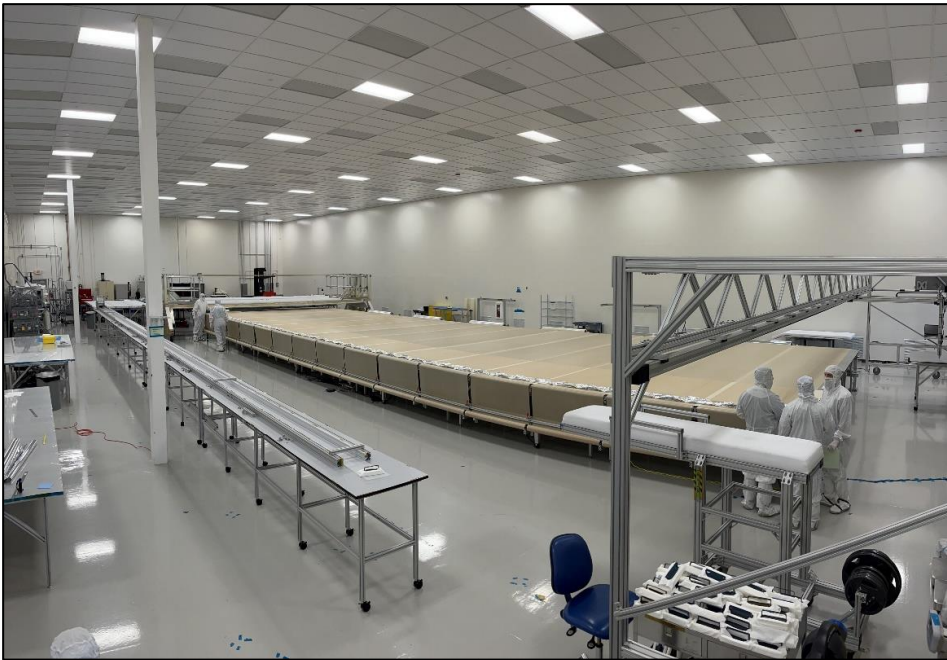
Folded Prototype SQ in spooling trough ready to begin spooling.
