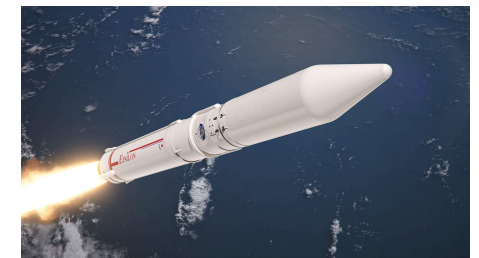
Epsilon launch vehicle (solid rocket engine)
