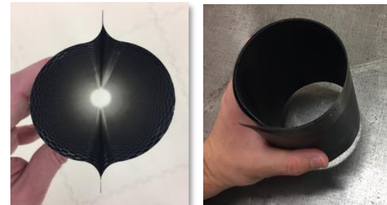
DCB 16.5-m boom cross section
