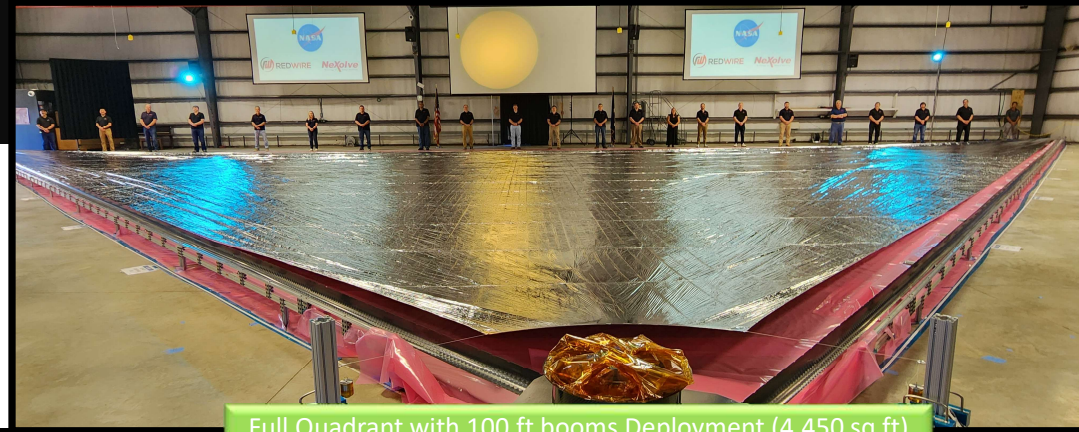
Full Quadrant with 100 ft booms Deployment (4,450 sq ft)
