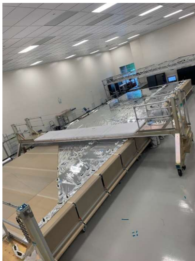
Prototype Sail Quadrant (SQ) Manufacturing
