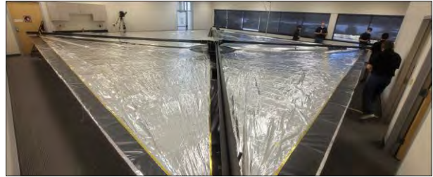
Fig. 4. Quarter-scale sail deployment test.
