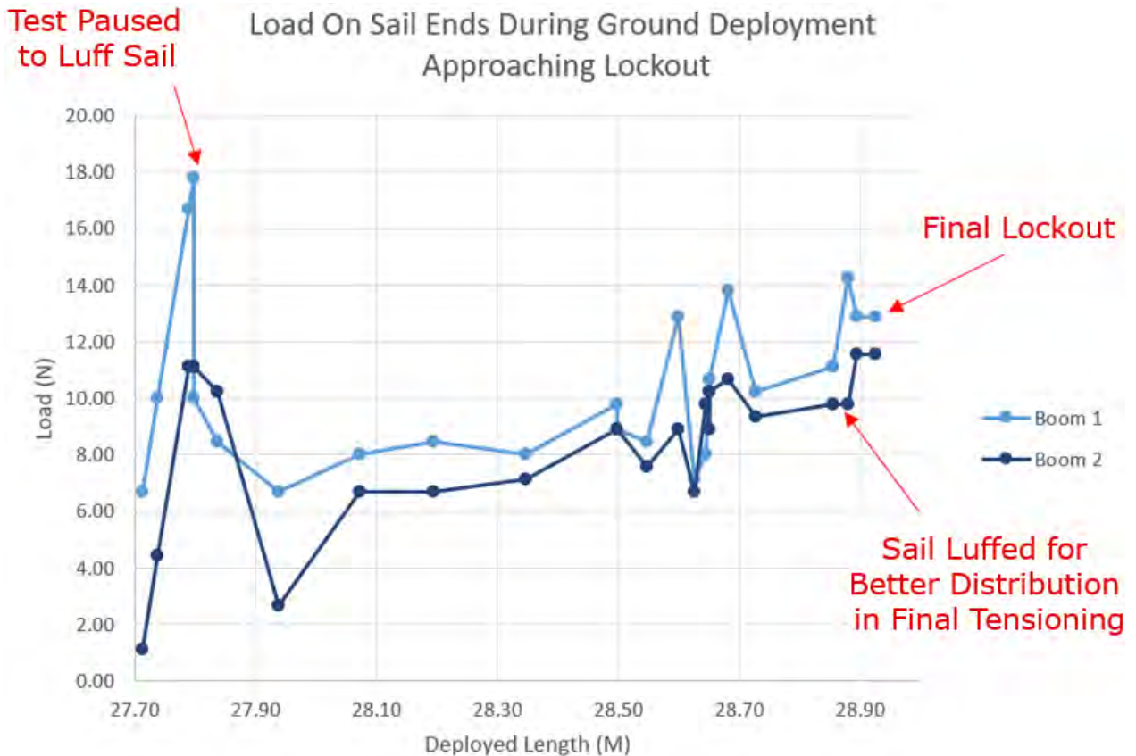
Fig. 6. Loads on sail ends during the final few meters of deployment, with some key events labelled in red.
