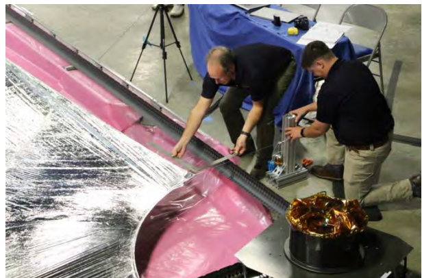
Fig. 8. Sail root cross-tie simulators being installed to tension the sail quadrant.
