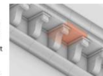
Cornice Underside 22/75 cracked 52/75 spalled / severely cracked 1/75 missing
