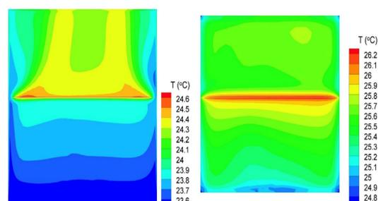
**Figure 1.** Temperature distribution on the wall with the crack: (left) outside surface and (right) inside surface. (Adapted from 2)
