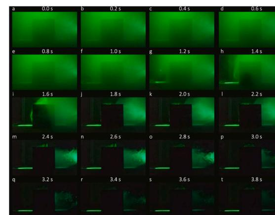
**Figure 2.** Flow visualization in the vertical center plane parallel to the wind flow from the side view. (Adapted from 5)
