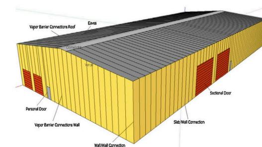
**Figure 3.** Relevant leakage of building component and connection of the sample building. (Adapted from 3)
