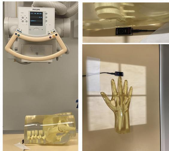
Figure 3: 1<sup>st</sup> image shows Lumbar spine positioning with the x-ray tube. Second image shows right hand in PA position with the Pascal dosimeter. Third image shows a close-up of Pascal dosimeter by lumbar spine.
