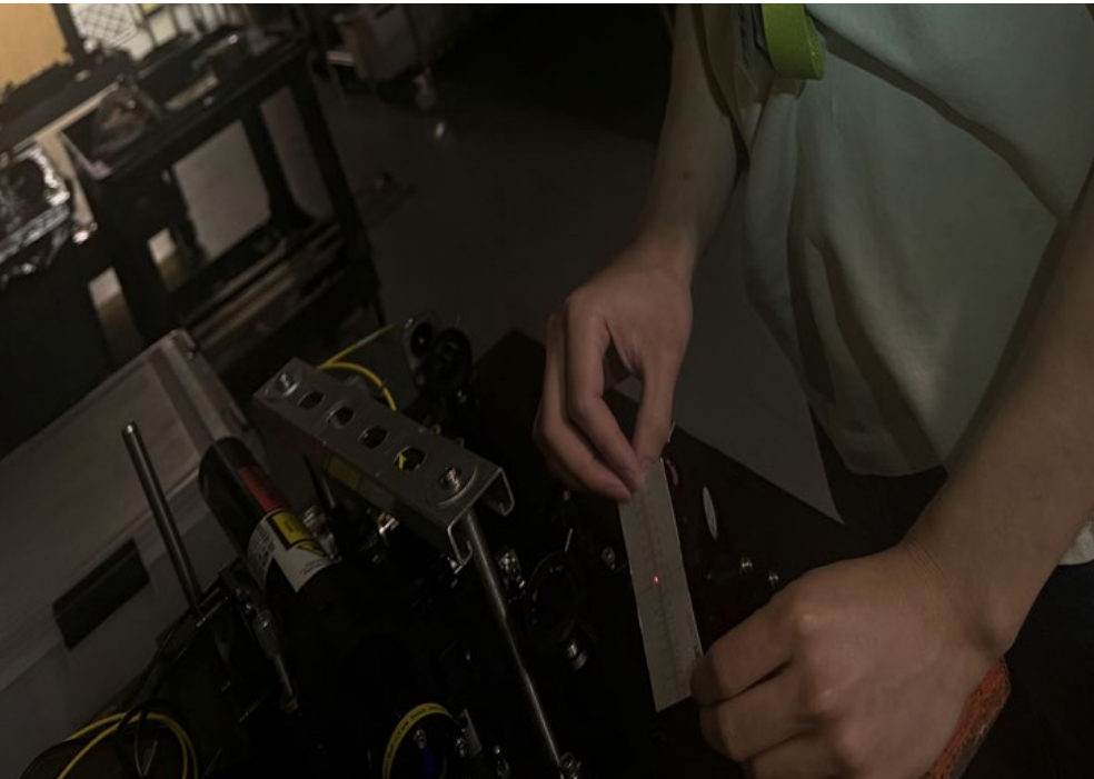
Alignment of a laser beam into a fiber optic cable
