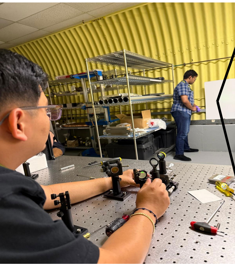
Precise alignment of optical components on an optical table for accurate laser beam delivery and magnification of a diffraction slide
