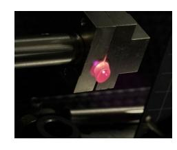
Ti:Sa is the crystal of choice for NIR UFHP lasers around the world due to its ability to lase in a very wide band centered at 800nm.
