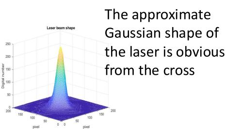
Laser beam quality is assessed and the fluence is calculated based on Beam spot size and beam energy on the sample
