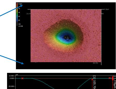
Nonlinear crystal used in Optical Parametric Amplification (OPA). Material defects lead to nonlinear damage effects.
