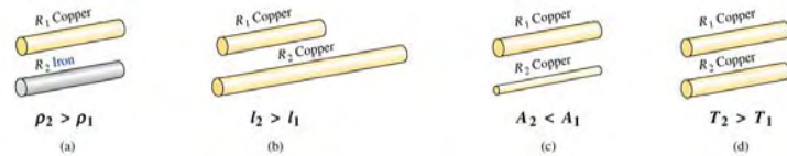
FIGURE 1.3 Cases in which R_2 > R_1 . For each case, all remaining parameters that control the resistance level are the same.
