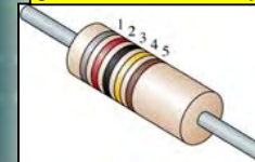
FIGURE 1.6 Color coding of fixed molded composition resistor.
