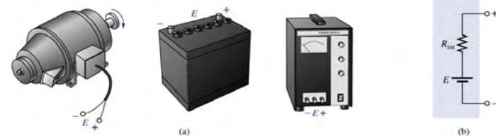
FIGURE 5.41 (a) Sources of dc voltage; (b) equivalent circuit.
