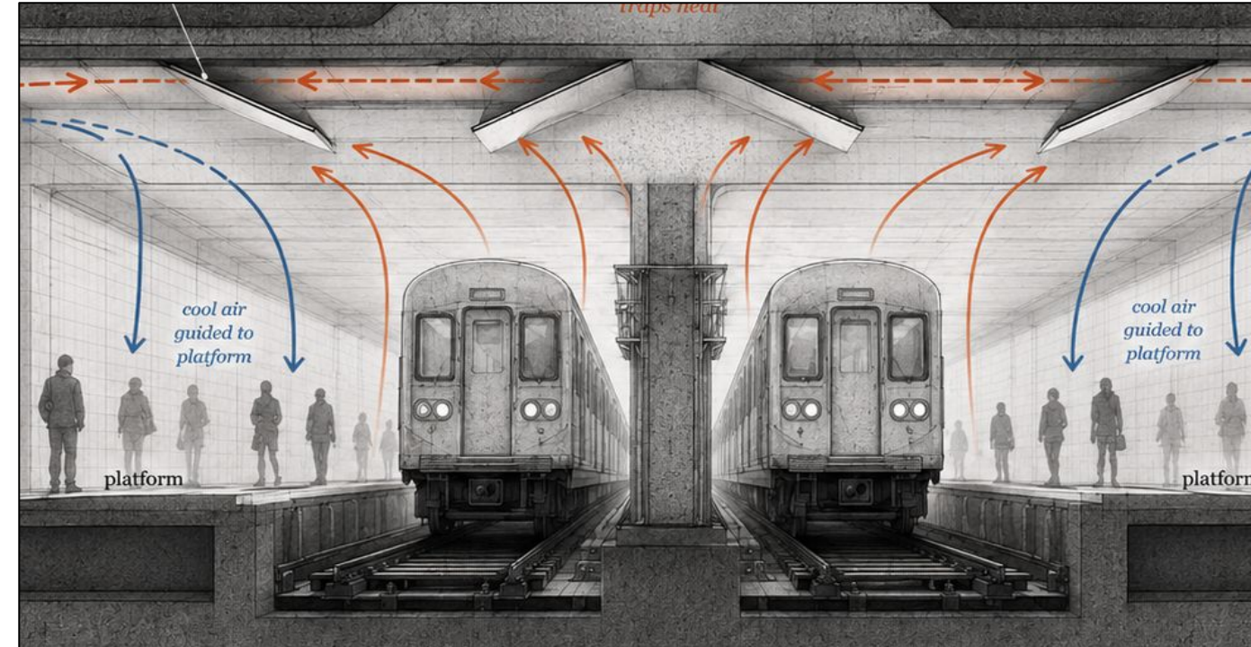
FIG 4.4 Angled Ceiling Deflectors Add passive angled panels to the low platform ceiling to push trapped hot air toward exhaust paths and guide cooler tunnel air down to passengers. Designed by student researchers via Adobe Illustrator and Enhanced using ChatGpt
