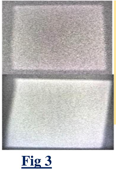
PDMS + 0.2 % SiC (top) low x-ray techniques (40kV, 1 mAs), and (bottom) is medium power X-ray 45kV, 10 mAS, no grid, 10 magnification). Low power x-ray image appears noisy (quantum mottle).
