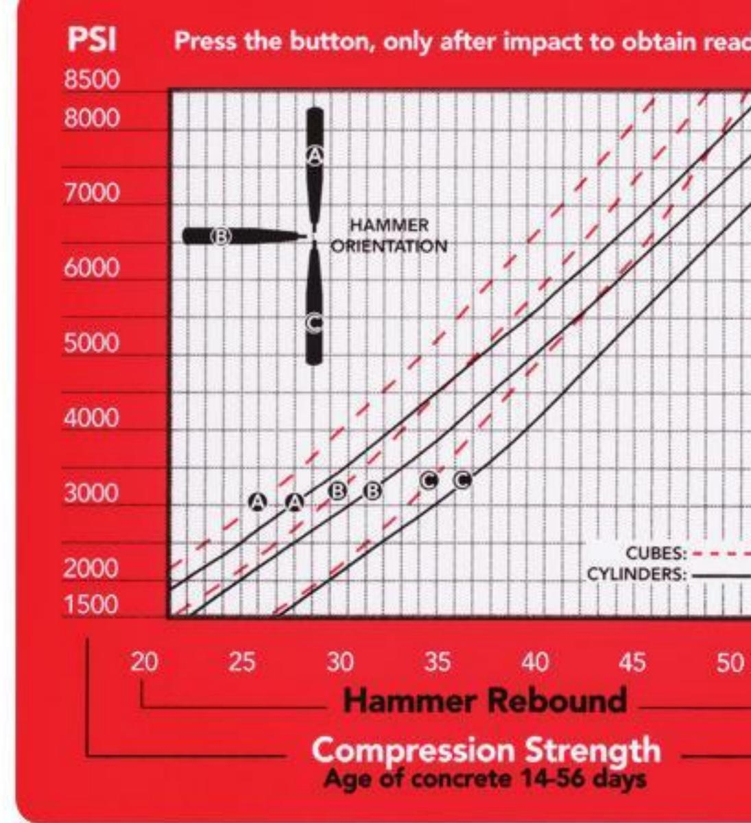
Depending on the position in which the test was taken, in this case Class A, the hammer rebound helps to determine the compressive strength in either PSI or MPa.
