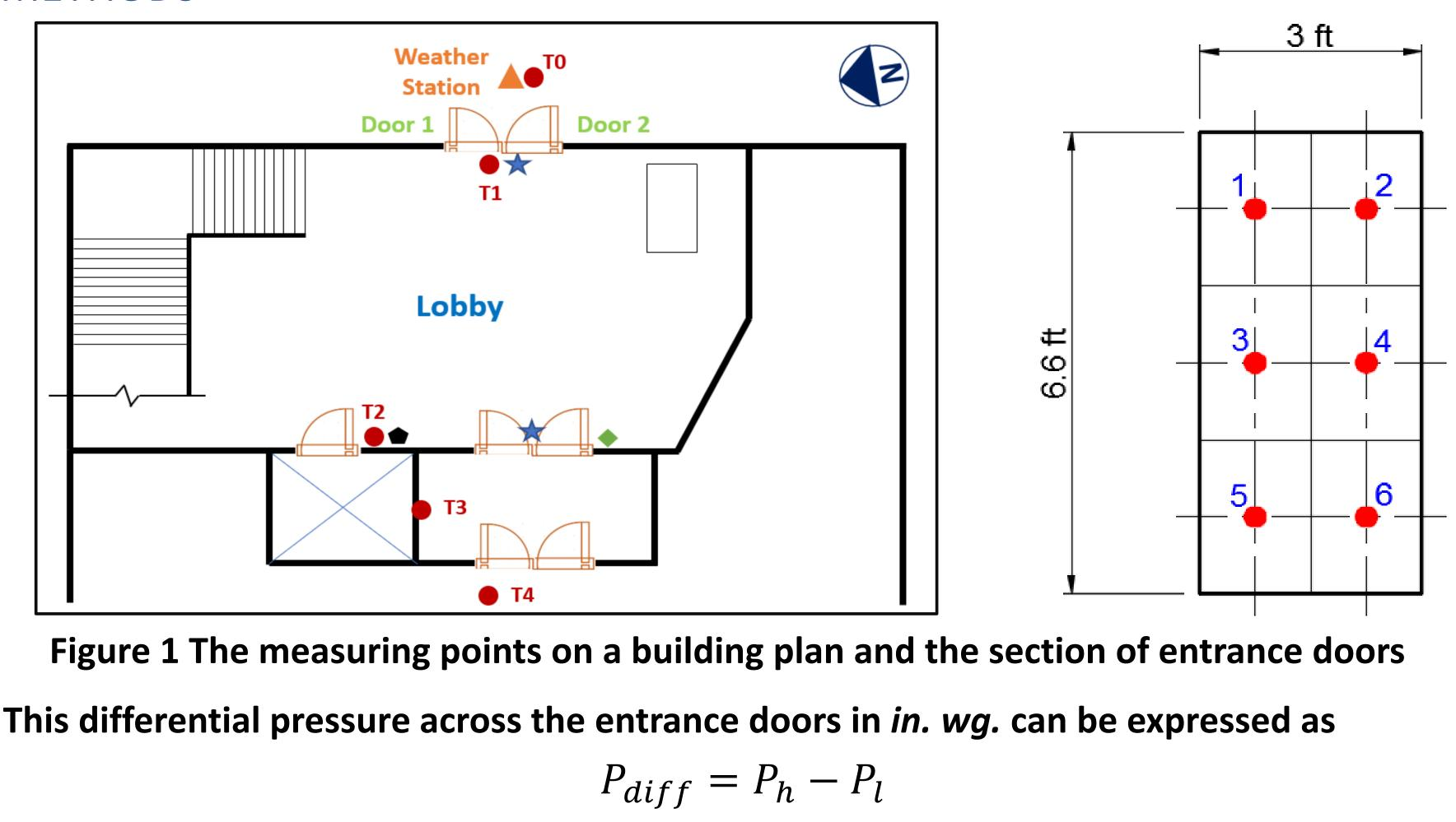
where  $P_h$  is high-pressure side in *in. wg.* and  $P_l$  is low-pressure side in *in. wg.* The air flow rate in CFM across the entrance doors is expressed as
