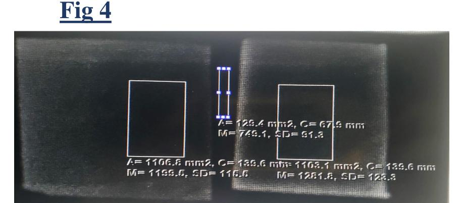
X-ray images of 0% SiC/polymer is shown on the right and 0.9% of SiC/polymer is shown on the left. Absorbed x-ray intensity and background noise are shown in the ROI's.
