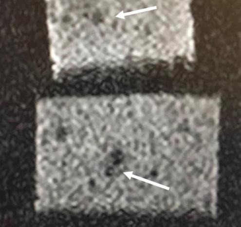
200 um resolution MR image (from Prisma 3T) Of 0% SiC/PDMS (top); 0.9% SiC/PDMS (bottom). Defects (white arrows) are approximately 1-2 mm in size (1000-2000 um)
