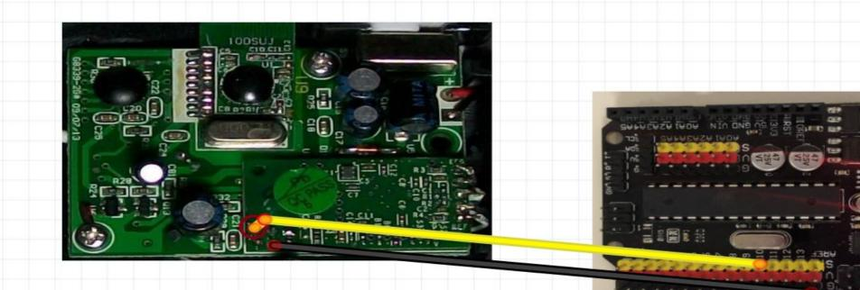
the yellow line: TX(mindflex)--->pin10 (Arduino) the black line: GND (mindflex) to the GND (Arduino)
