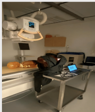
Figure 6: Parent shielded and 1 foot away from the edge of the exposure field.
