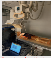
Figure 3: X-ray tube positioned 40 inches SID. The child is positioned AP chest (back towards the image receptor). The parent is 1 foot away from the edge of the collimated field. The pascal dosimeter and computer is placed on the cart next to the parent to record dose.
