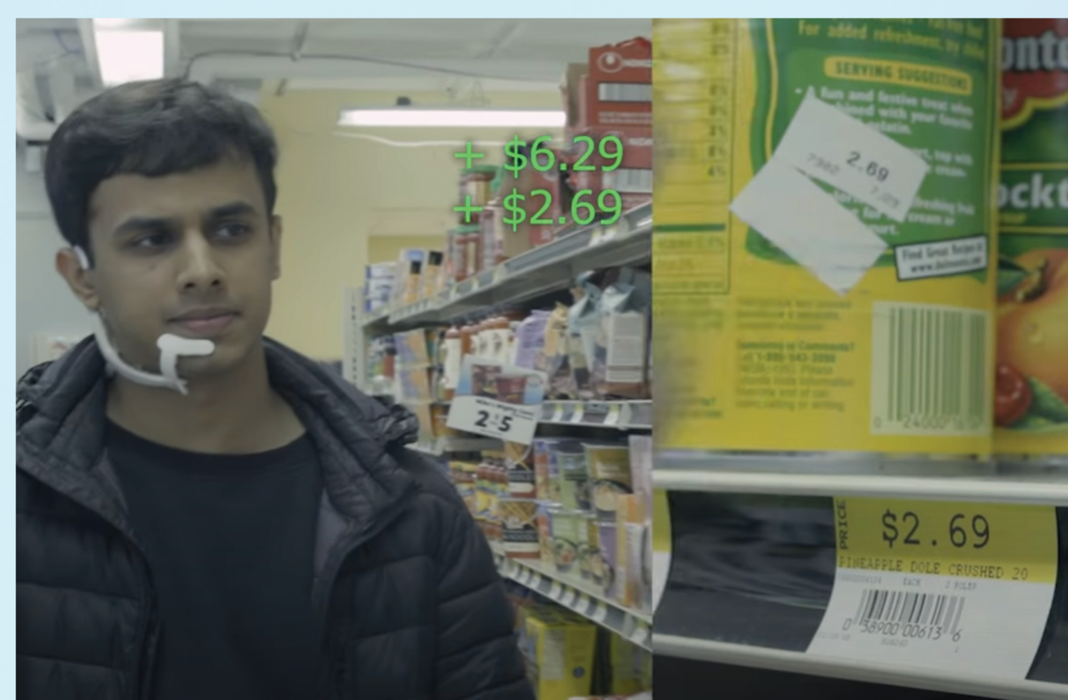
Fig. 1: "AlterEgo is a wearable system that allows a user to silently converse with a computing device without any voice or discernible movements."
