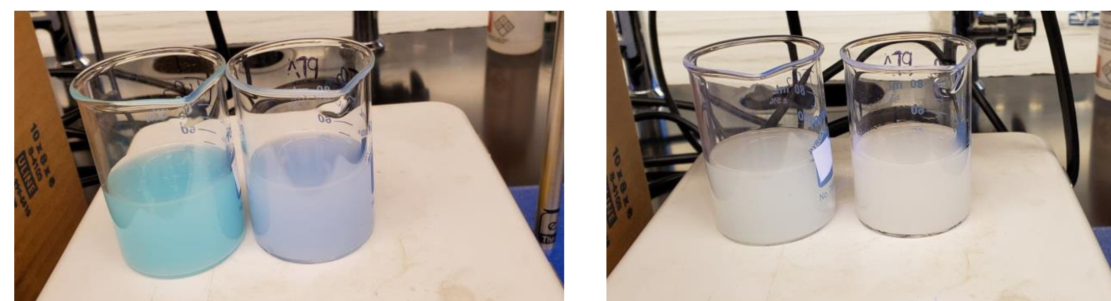
Fig 3. Low concentration of MB with \text{TiO}_2 (left) and \text{TiO}_2 + \text{PTA} (right) under UV light; the MB has significantly degraded over time.
