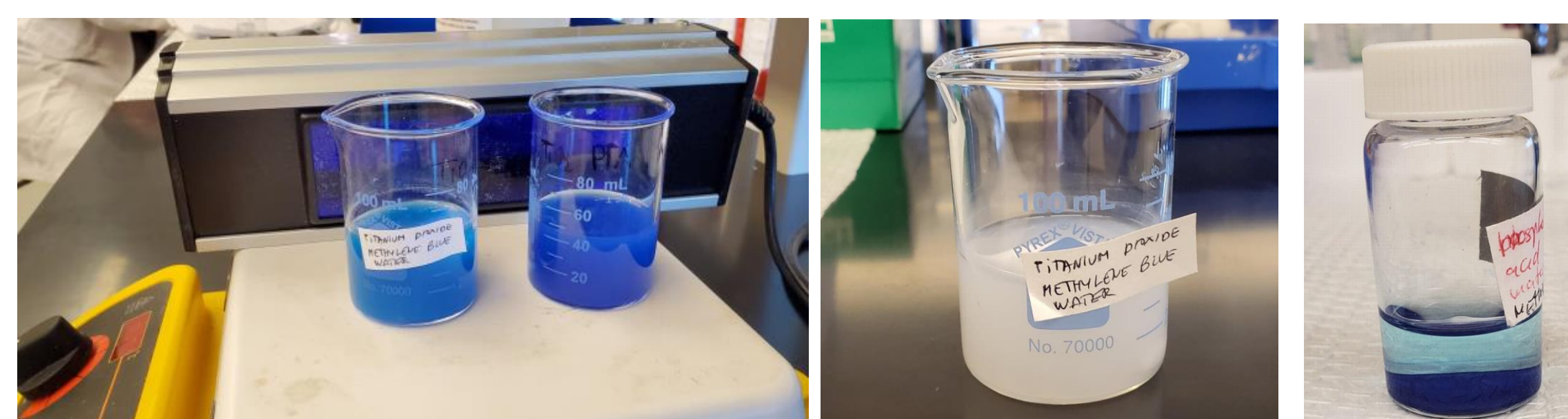
Fig 2. High concentration of MB with \text{TiO}_2 (left) and \text{TiO}_2 + \text{PTA} (right) under UV light; MB has not degraded completely with \text{TiO}_2 -PTA.
