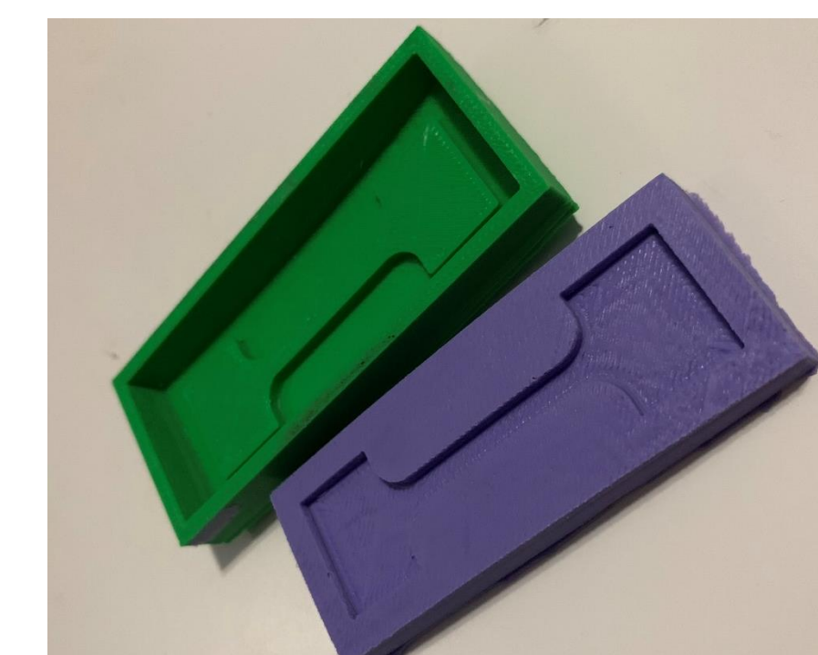
Fig 4. 3D printed Dog-Bone and silicone molds
